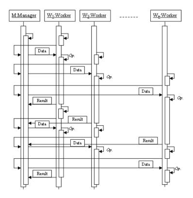
Fig. 2. Interaction Diagram of the Manager-Workers pattern.
