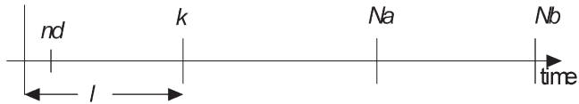
Fig. 6 Time horizons with respect to time delays, horizon samples, and k sampling time
