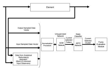
Fig. 2.1 Process diagram for Fault Localization
