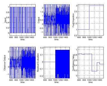
Fig. 4.3 Fault and Fault-Free Scenarios with Residual Evaluation and Time Invariant Behaviour
