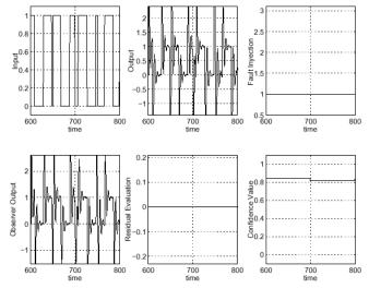
Fig. 4.4 Fault-Free Scenario with Time Variance Input Behaviour with Residual Evaluation
